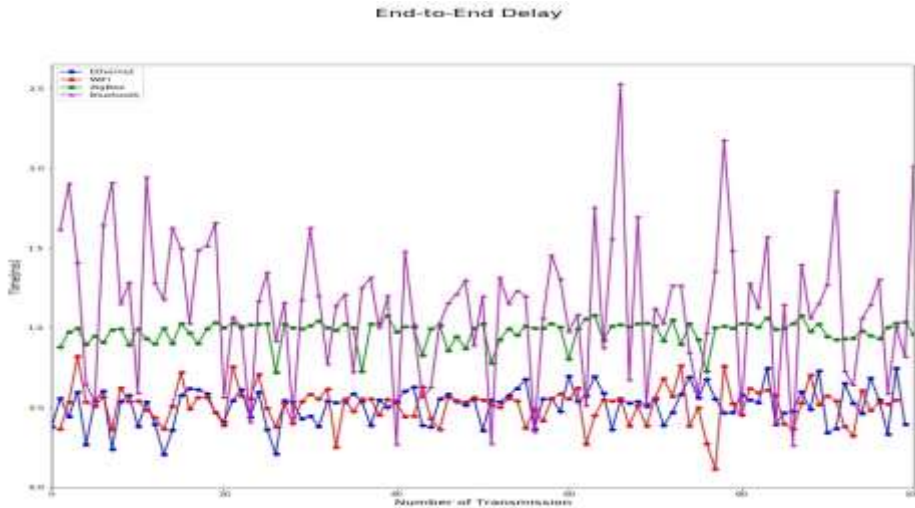
Figure 21: End-to-end delay of Ethernet, Wi-Fi, Zigbee and Bluetooth communication
