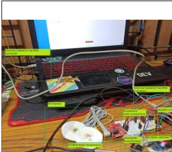
Figure 10: Connection of the working prototype with Ethernet Cable(CAT 5e)
