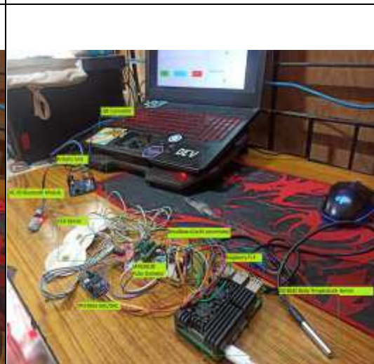
Figure 13: Bluetooth module (HC-05) with Arduino Uno and Raspberry Pi
