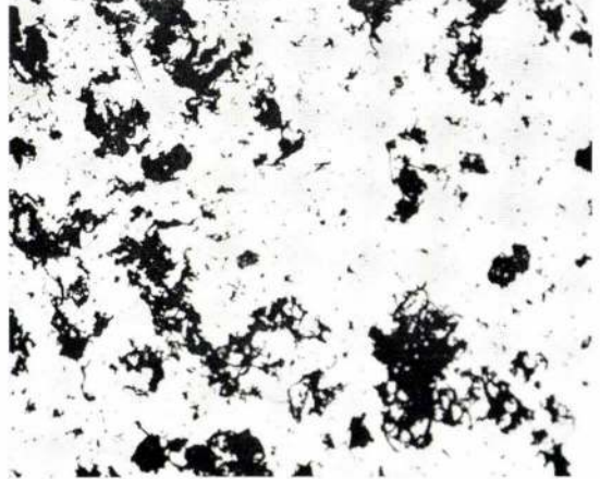
Photo. 9. Marcona pellet (CO 100 cc/min, 900°C, 4 hr) ( \times 100 ) (2/3)
