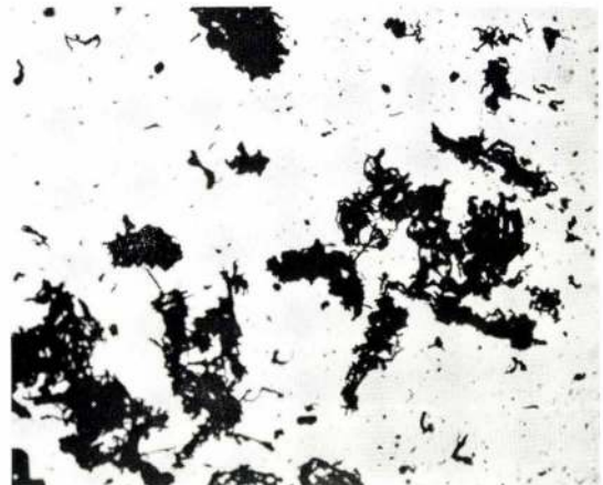
Photo. 4. Marcona pelletizing feed (CO 200 cc/min, 900°C, 5 hr) ( \times 100 ) (2/3)
