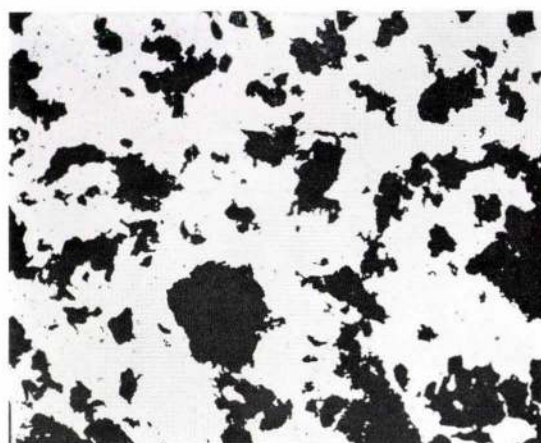
Photo. 18. Marcona pellet (H 2 100 cc/min, 1 100°C, 4 hr) (×100) (2/3)
