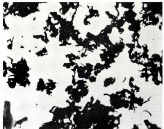
Photo. 5. Marcona pelletizing feed (CO 200 cc/min, 1 000°C, 5 hr) ( \times 100 ) (2/3)
