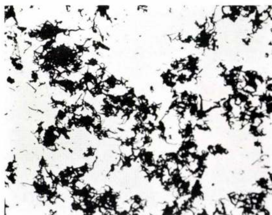
Photo. 17. Marcona pelletizing feed under 325 mesh (CO 200 cc/min, 900°C, 5 hr) (×100) (2/3)
