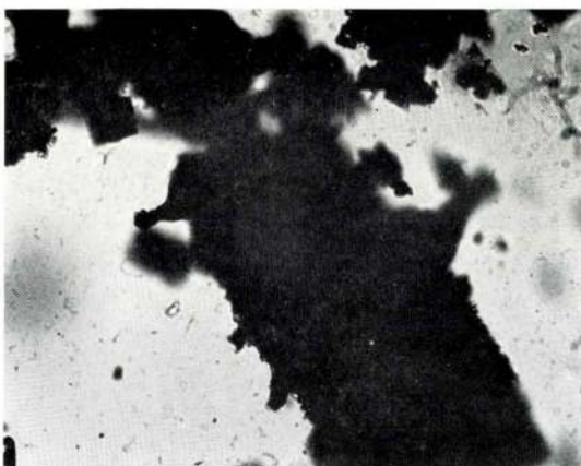
Photo. 12. Marcona pelletizing feed taken from bottom layer (CO 200 cc/min, 900°C, 1 hr) (×100) (2/3)
