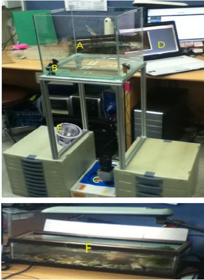
Fig. 3. A (transparent aquarium), B(diving beetles), C(a high speed camera), D(a laptop computer), E(a lamp), F(a residential aquarium). An Experimental environment has been set up to get the motion data of diving beetles (B) while they are swimming in a transparent aquarium (A). The recorded data by the high speed camera (C) is imported to a laptop computer (D). A lamp (E) was positioned on the ground to make video images clear
