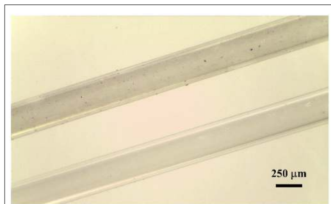
FIGURE 4 | Optical microscopy image of the pristine silica capillary before (bottom) and after (top) undergoing EPD using a MWCNT suspension as described in the Materials and Methods section. Note that the orange polyimide coating covering the outer surface of the capillary has been burned off.
