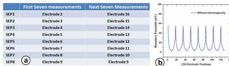
Fig. 6. (a) Symmetric electrode pairs (SEP) of a 16 electrode EIT system in current projection 1, (b) Boundary potentials for homogeneous medium.
