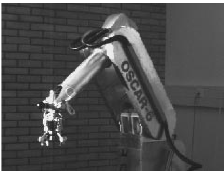
Figure 6.6: The OSCAR-6 robot arm. OSCAR is designed for pick-and-place tasks and has been applied in several industrial settings. The arm contains 6 total joints and a camera mounted in the end effector. This OSCAR-6 robot is owned by the Autonomous Systems Group at The University of Amsterdam. Printed with permission.
