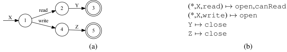
Fig. 5. (a) Symbolic automaton representing the query for the behavior around read and write methods and (b) the assignment with contexts to its symbolic transitions which answers the query.
