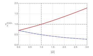
FIG. 4. Group velocity  $v_{\mathrm{g}(\pm)}$  [Eq. (113)] of d-transversal case. The blue dot-dashed curve indicates  $v_{\mathrm{g}(+)}$ , while the red solid line represents  $v_{\mathrm{g}(-)}$ . The vertical dashed line indicates  $|\tilde{\alpha}| = 1$ , corresponding to the value of the critical factor  $\alpha_c$  [Eq. (114)] for the choices  $\mu = 1$ ,  $\epsilon = 2$  and d = 1, the ones adopted in this plot.
