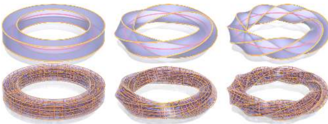
Fig. 13. We can allow the torsion of the frame along singular and feature curves to be free during optimization—and hence do not have to determine torsional periods a priori . Here for instance the frame automatically makes the correct number of twists as it travels around the red loop (from left to right: 0, 1, and 2), keeping it compatible with the boundary normals.
