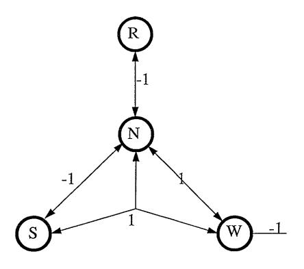
Figure 2: A cubic network that represents E = -NSW + NS + RN - WN + W using Sigma-Pi units and a cubic hyper-arc. (Its is equivalent to the network of Figure 1 without hidden units)
