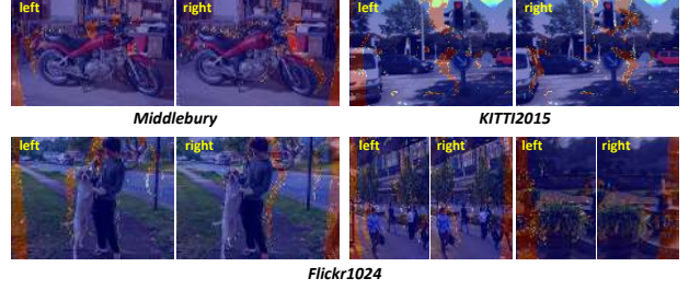
Figure 3: An illustration of valid masks generated by our occlusion handling scheme. Red regions have small values and represent heavy occlusions.
