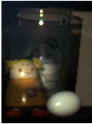
Figure 6: Relighting with 2 spot lights. Image rendered from a reflectance field captured by our system. The egg and the wooden toy are lit from 2 spotlights (with spatially varying intensity distribution), one shining from the right and the other from left. Another faint floodlight adds to the overall brightness of the scene. Note that the caustics from the glass, specularities on the egg, and the toy, and shadows are all faithfully reconstructed.
