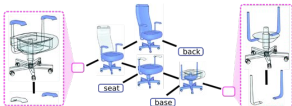
Figure 6: Unnatural hierarchy as a result of omitting certain precedence rules. The same node organization is obtained by omitting M2 or G2 . The zoom-ins reveal parts of the armrest that should be grouped but are separated, in contrast to the more natural result in Figure 2 (first chair).
