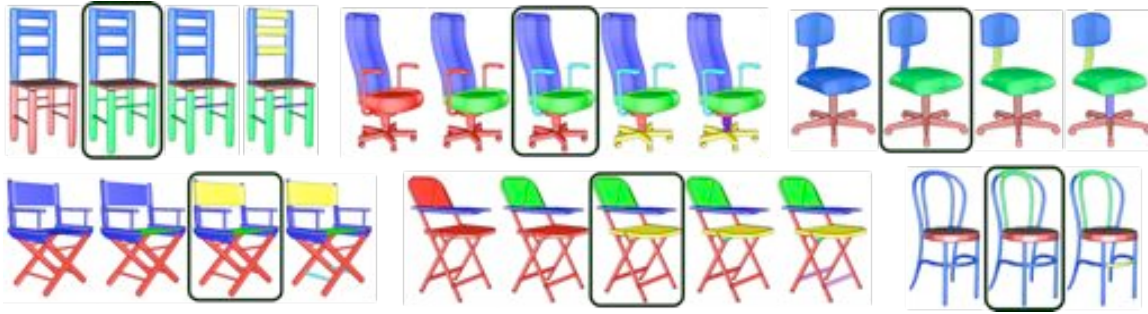
Figure 7: Hierarchical segmentations of several chair models. Results marked by boxes produce semantic parts: back, seat, legs, and armrests (if any), e.g., compare to the symbolic hierarchies shown in Figure 2. Note the imperfect result for the last chair as part of the back is not separated from the legs; this is due to the initial segmentation unable to do so (see Figure 3).
