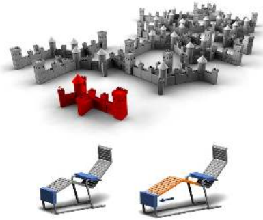
Figure 23: Inverse procedural modeling from symmetry: By attaching building blocks derived from boundaries between non-symmetric area (docking sides), shape variations can be created automatically (top; original in red). Sliding dockers (bottom, orange) generalize the idea to partial patterns.
