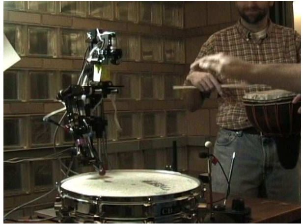
Fig. 1. Nico, drumming in concert with human performers. The robot responds to both visual and auditory stimuli from its human concert partners in order to produce the appropriate, correctly phased tempo.
