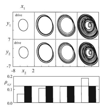
FIG. 7. In the first two panels, the attractors of Eq. (11) are shown as  $\rho$  is varied in the drive through several bifurcations and the response follows, despite its  $\rho$  being held constant. The third panel shows the change in the drive bifurcation parameter (white bars), but the response parameter (black bars) is held constant (from Ref. 22).
