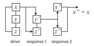
FIG. 4. A schematic in how to set up a cascaded drive-response system that reproduces the original drive signal. Note this is only possible when the two different response systems are stable to their drive signal. For example, it is possible with the Lorenz system above, but not the Rössler system.
