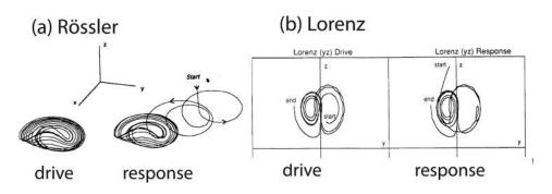
FIG. 3. Rössler and Lorenz driveresponse systems. (a) The Rössler ydrive-response system of Eq. (5). The y-component is the same in both drive and response systems. The systems are started out of sync, but the response soon spirals into an attractor synchronized with the drive. (b) The Lorenz x-drive-response system of Eq. (3). (Adapted from Refs. 3 and 4)
