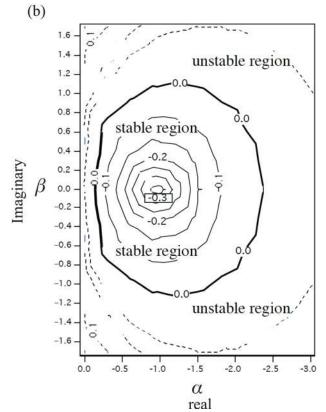
FIG. 10. Plots of the master stability function in the case of (a) symmetric coupling matrices (real eigenvalues) and (b) nonsymmetric coupling matrices (complex eigenvalues, in general) for *x*-coupled Rössler networks (from Refs. 23 and 61).
