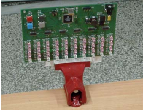
Figure 2 A PCB board based on DSP (MicroChip) embedded microprocessor with LEDs
