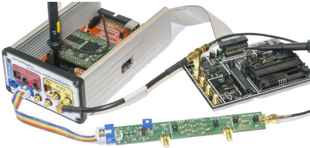
Fig. 18 Test Setup for side-channel analysis with clock recovery of internal oscillator on ATMega48A. The oscilloscope is used to measure recovered clock frequency. The long board center-front performs amplification, filtering, and limiting. The PLL is located inside the capture hardware on the left-hand side. The back right board is the AtMega48A target.
