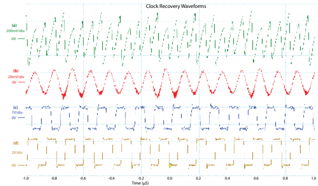
Fig. 15 Recovery of 7.7 MHz Internal RC Oscillator on AT-Mega48A. (A) is the amplified power trace after the LNA. (B) is the output of the band-pass filter, and (C) is the output of the limiter, which generates a logic-level signal. The output of (C) can be passed through a PLL to further stabilize the signal. In (D) the actual RC oscillator output is shown, note the perfect alignment of the recovered clock (C) and internal RC oscillator (D).
