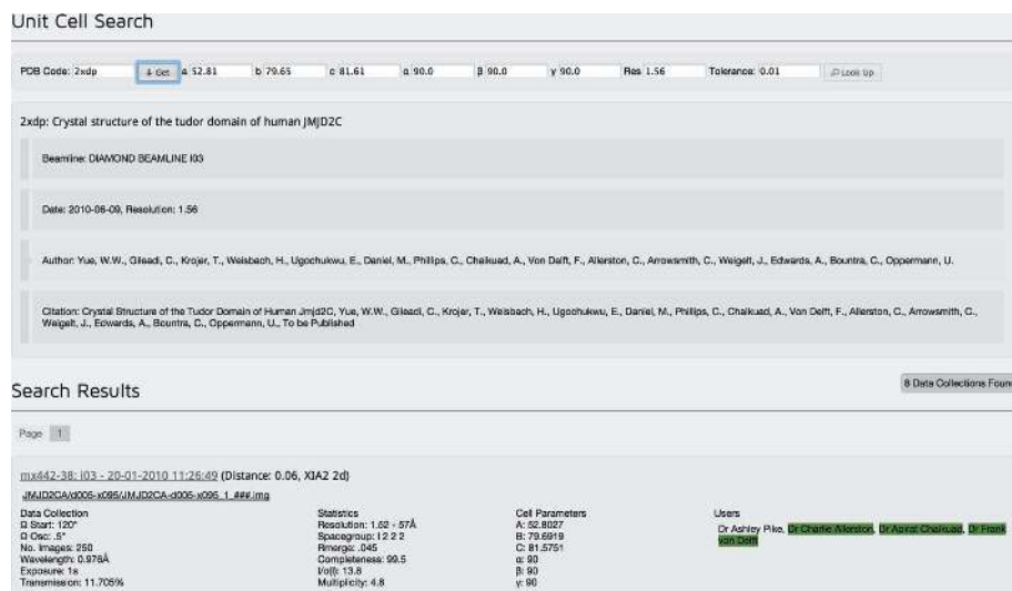
Figure 8 Unit-cell search, here showing auto-processing results related to PDB entry 2xdp. Authors registered on the visit that match the PDB file are highlighted in green.
