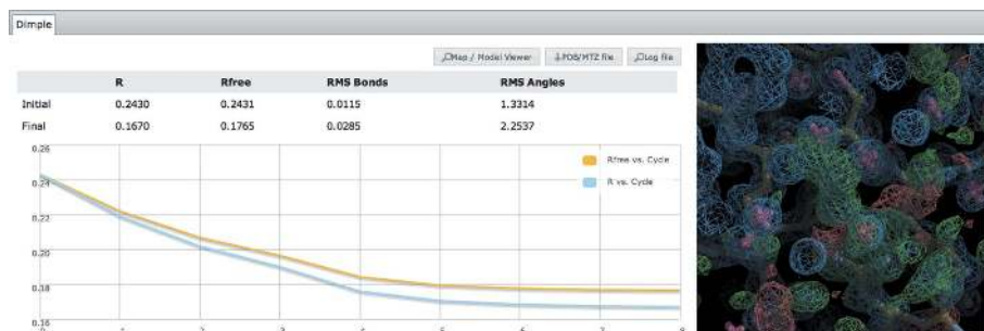
Figure 5 Results from DIMPLE showing cycle versus R factor and DIMPLE 'blob' images showing regions of unmodelled density. Here the bound tartaric acid in thaumatin is clearly visible.
