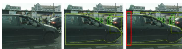
FIGURE 4. Examples of visual comparison on the Cityscapes dataset. To show the effect of Syncretic-NMS more clearly, the example image is a screenshot of the original image. The three columns of the image from left to right are a screenshot of the original image, the prediction result of Mask R-CNN, and the prediction result after using Syncretic-NMS. The red area in the figure is the enlarged range of the bounding box, which was manually labeled.
