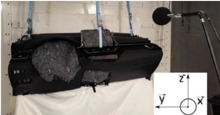
Fig 36. The usage of noise absorber which investigated by Bennouna et al. [75]
