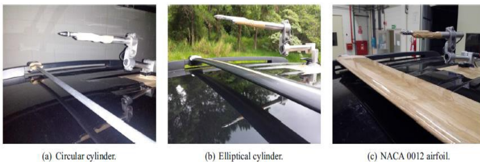
Fig 47. Crossbar profiles configurations which investigated by Massarotti et al [63]
