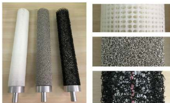
Fig 12. Different porous cylinder studied by Arcondoulis et al. [38]
