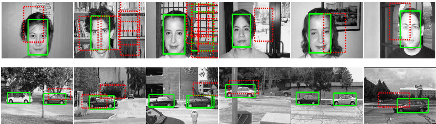
Fig. 12: Sample detection results on the datasets of [1], [14]. The locations proposed by a bottom-up detection system are used to initialize an EM-loop which brings in additional information from segmentation and the AAM parameters. Based on these, the initial hypotheses are either pruned (red dashed boxes) or validated (green boxes).
