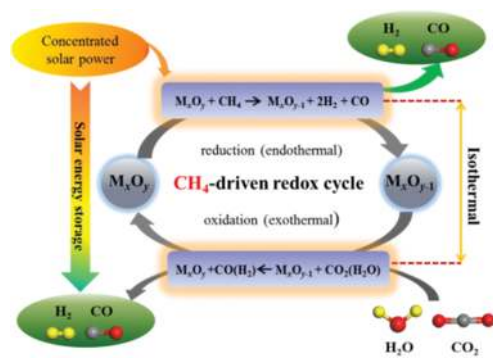
Fig. 1 Schematic of two-step solar thermochemical carbon dioxide splitting and water splitting processes coupled with methane driven reduction (MDR-STCDS, MDR-STWS).
