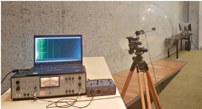
Fig. III.1: Extracting an image from a screen using a parabolic microphone at a distance of approximately 5 meters.
