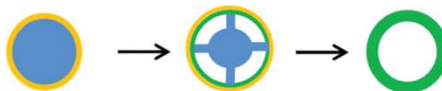
Fig. 9 Hollowing by the Kirkendall effect.
