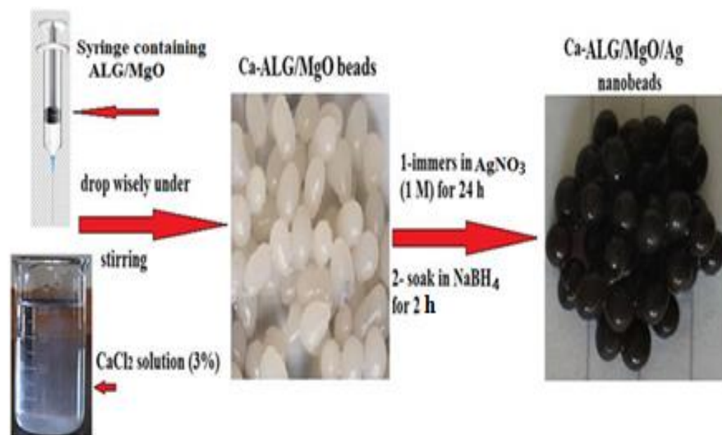
Figure 12. Steps of preparation of Ca-ALG/MgO/Ag nanocomposite beads supported with digital photos.
