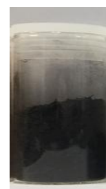
Figure 8 Rice husk ash (RHA) obtained after 400 °C heat treatment.
