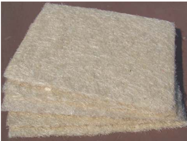
Figure 3. Sisal preform made up of chopped sisal fibre length of 5 cm.
