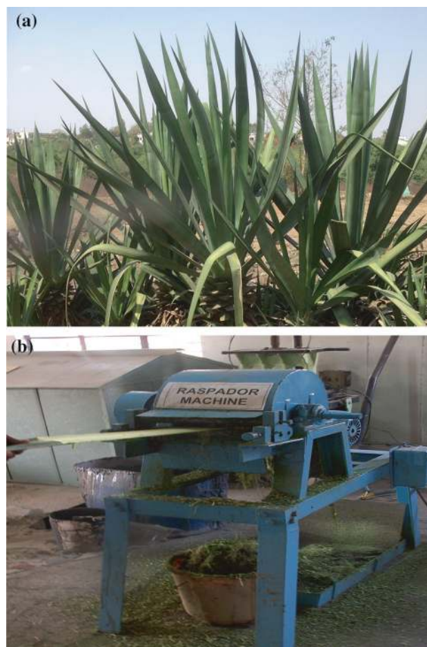
Figure 1. (a) A fully grown up sisal plant after five years of plantation. (b) Sisal fibre mechanical extraction process.
