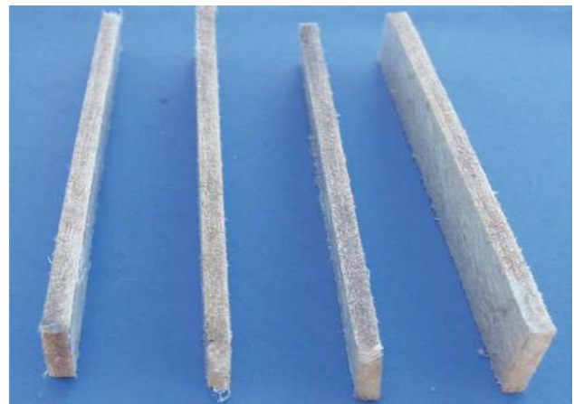
Figure 6. Samples of sisal preform composites made up of chopped sisal fibre length of 5 cm used for testing tensile strength and impact studies.
