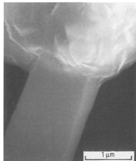
Figure 7 SEM micrograph showing a polycrystalline granule at the root of a \beta' -sialon whisker.
