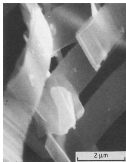
Figure 9 SEM micrograph of \alpha\text{-Si}_3\text{N}_4 whiskers with NaF as molten bath.
