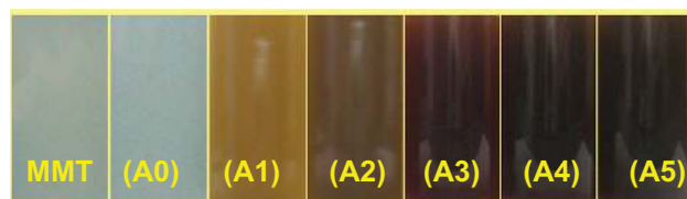
Figure 2 Photograph of montmorillonite/chitosan bionanocomposite suspension (A0) and silver/montmorillonite/chitosan bionanocomposite suspension at different \text{AgNO}_3 concentrations; (A1) 0.5%, (A2) 1.0%, (A3) 1.5%, (A4) 2.0%, and (A5) 5.0%.
