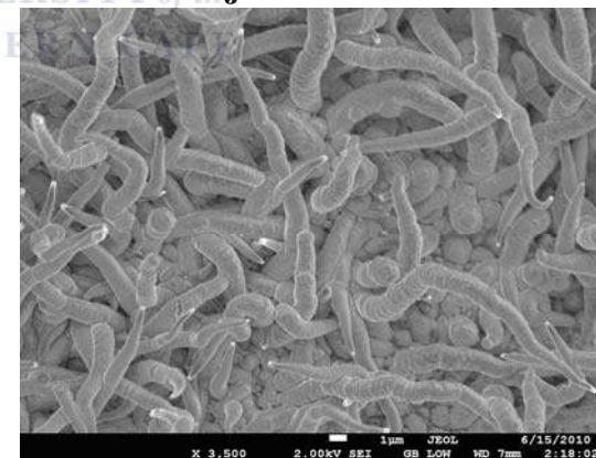
Figure 4.4: SEM images: (G) electrochemically polymerized G2PPI-co-PPy ( \times 3500 ), (H) electrochemically polymerized G2PPI-co-PPy ( \times 10,000 ), (I) electrochemically polymerized G3PPI-co-PPy ( \times 2000 ), (J) electrochemically polymerized G3PPI-co-PPy ( \times 10,000 ), (K) electrochemically polymerized G4PPI-co-PPy ( \times 3500 ), and (L) electrochemically polymerized G4PPI-co-PPy ( \times 3500 ).
