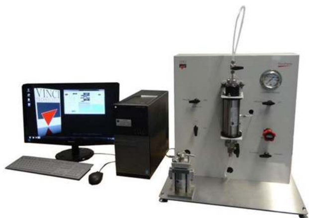
Fig. 6 Vinci technologies steady-state gas permeameter (Gasperm)
