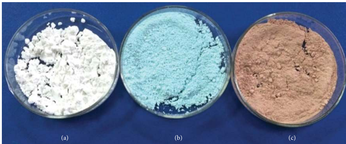
FIGURE 1: Photograph of zeolite (a), \text{Cu}^{2+} /zeolite (b), and \text{Cu}_2\text{O} NPs/zeolite (c).
