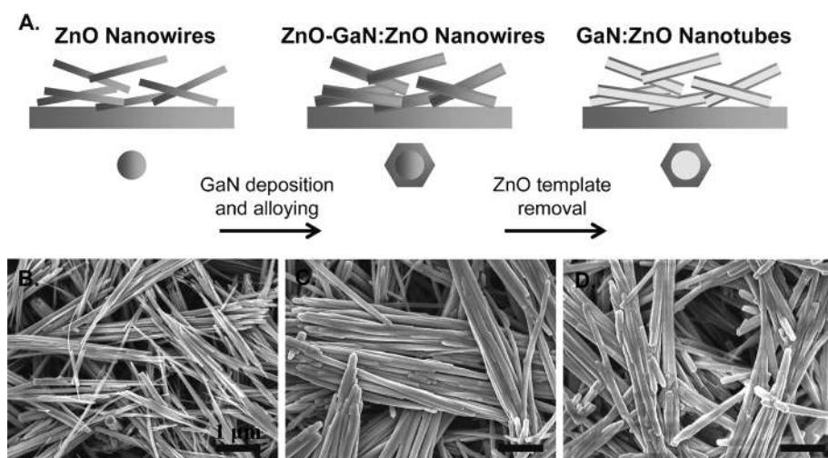
Figure 1. A) Schematic showing the epitaxial casting procedure used to generate GaN:ZnO nanotube films. B–D) SEM images of films consisting of B) ZnO nanowires, C) ZnO-GaN:ZnO core-shell nanowires, and D) GaN:ZnO nanotubes.
