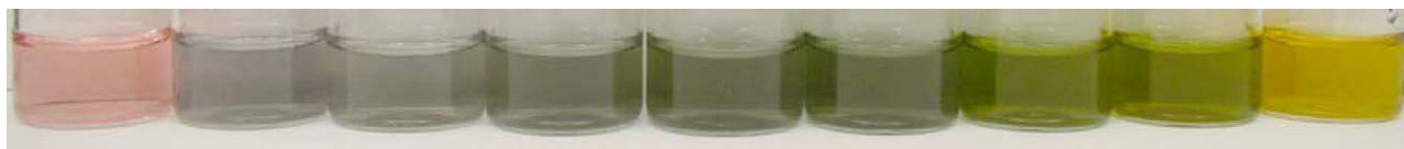
Fig. 17. Gold core–silver shell particles that absorb various wavelengths of light (the eight vials on the right), compared to gold colloid (far left).
