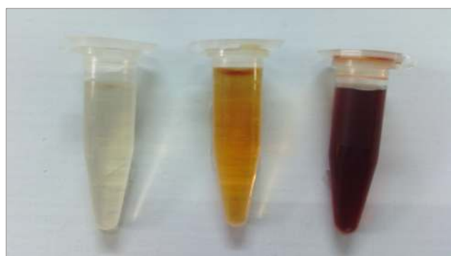
Figure 1: Optical Photograph of (a) AgNO 3 solution, (b) A. grandiflora extract and (c) AgNPs solution.
