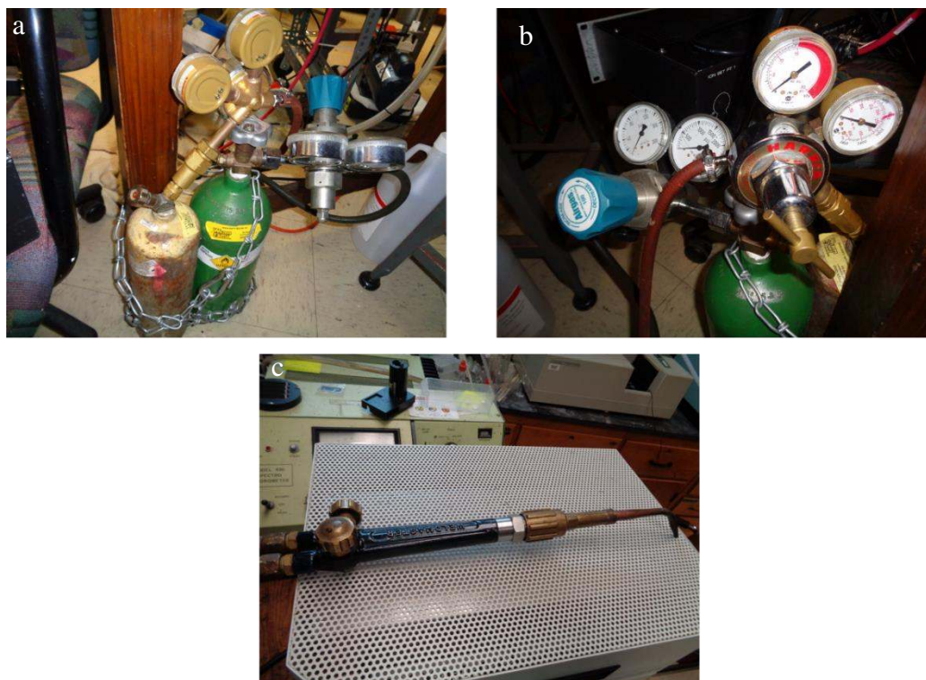
Figure 2.8 a.) and b.) Oxygen and acetylene tanks used for glass sealing. c.) Oxy-acetylene torch
