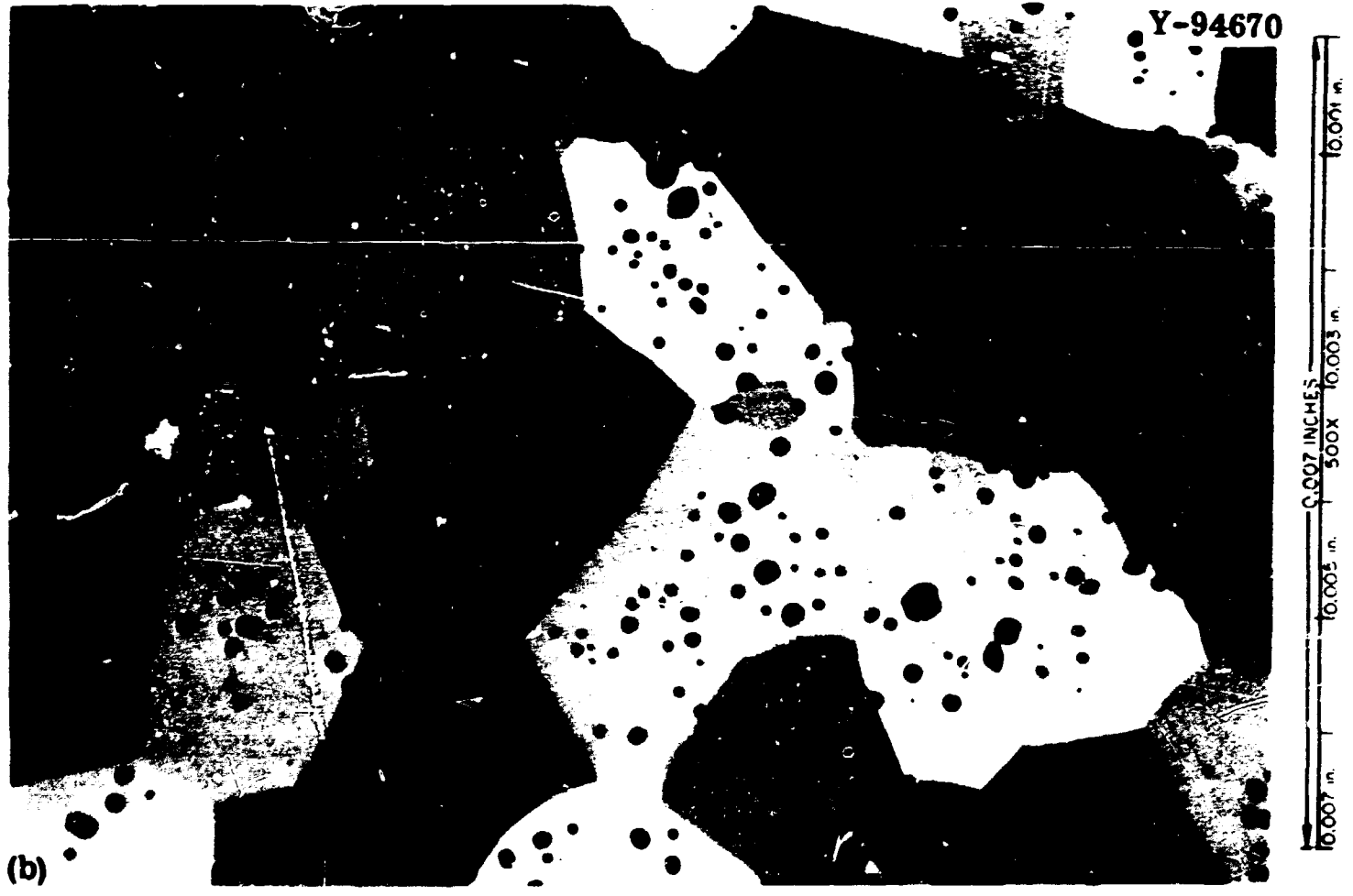
Fig. 21. Microstructures of UN Specimens (a) R470 and (b) R471.
