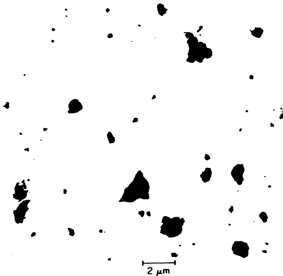
Fig. 8. Electron Photomicrograph of UN-5 Particles After Spatulation.
