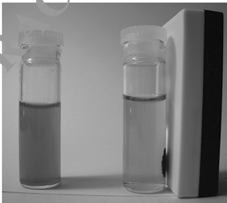
Figure 3 Magnetite-hexane suspension attached to a magnet.
