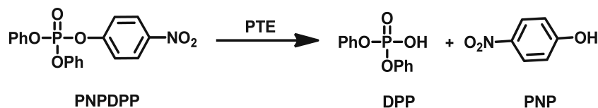
Scheme 3. Hydrolysis of phosphotriester (PNPDPP) to diphenylphosphate (DPP) and p -nitrophenol (PNP) in the presence of PTE.
