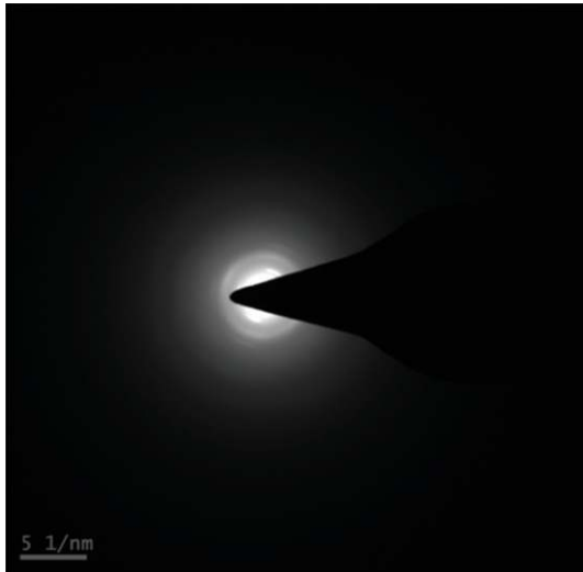
FIGURE 3: SAED patterns of prepared ZnO nanopowder.
