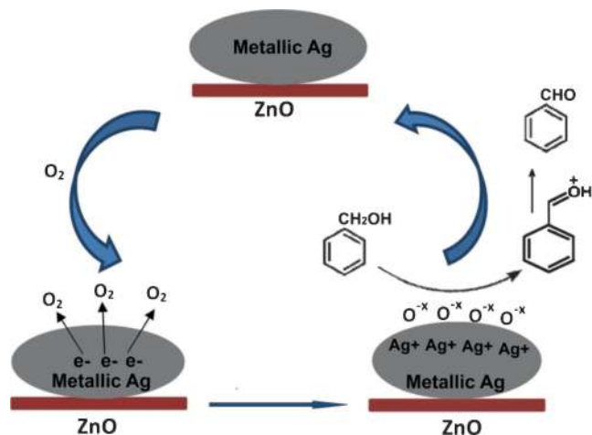
Scheme 1. Schematic reaction mechanism of benzyl alcohol oxidation on Ag-ZnO nanocomposite.
