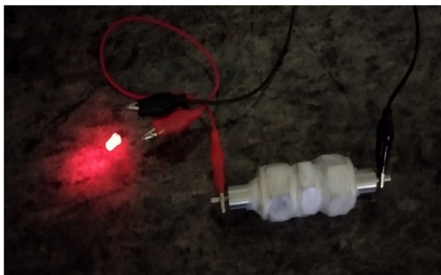
Fig. 11 Swagelok cell illustrating the working of red LED-after charging for 10 minutes, after 8 minutes, intensity started to diminish.
