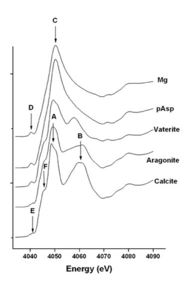
Fig. 2. X-Ray absorption spectra showing pre-edge and XANES regions of calcite, aragonite and vaterite reference samples, and samples of ACC produced using 9:1 Mg:Ca (isolated after 240 min) and 100 µg ml-1 pAsp (isolated after 50 min).
