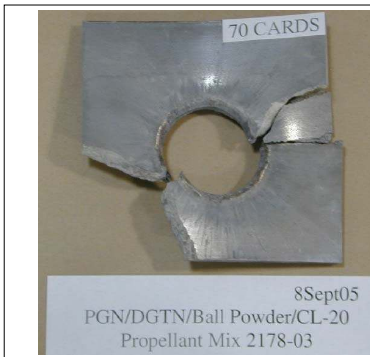
Figure 5—13. Result of NOL LSGT at 70 cards. Result is “GO”.
