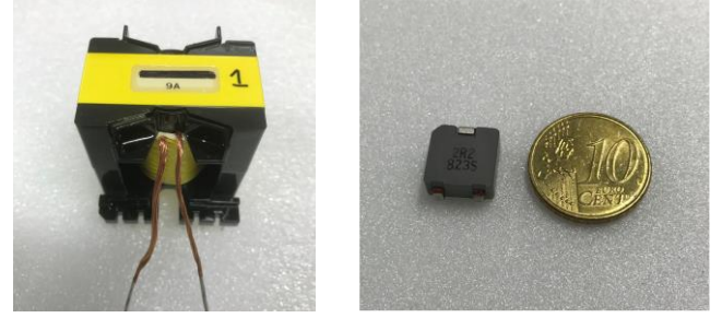
(a) Reactor with 10-turn litz wire (b) Power inductor [28]
