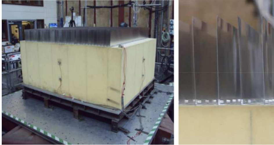
Fig. 9 Left: shaking table (Bristol Laboratory for Advanced Dynamics Engineering) equipped with aluminum sheets acting as resonators as studied in Ref. [277]; right: zoom on the sheets (original pictures by Professor Claude Boutin)
