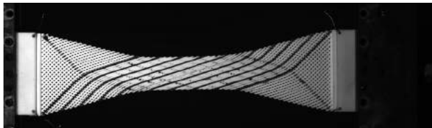
Fig. 22 A pantographic sheet under extensional bias test as studied in Ref. [358]: a concept for a new lightweight, extremely resistant and safe in failure architected material (original picture by the authors)
