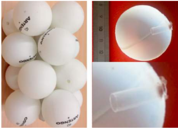
Fig. 7 Another example of handcraft metamaterial: hollow plastic spheres (138 mm high) with a central impervious cylinder studied in Ref. [276]. Spheres might be impervious hollow spheres, or resonators, or both (see Table 1 in the reference paper for details). The interspheres space might be occupied either by air or filled by a granular medium. Left: geometry of the prototype; middle: a prototype; right: cut of the two types of Helmholtz resonators (original pictures by Professor Claude Boutin).
