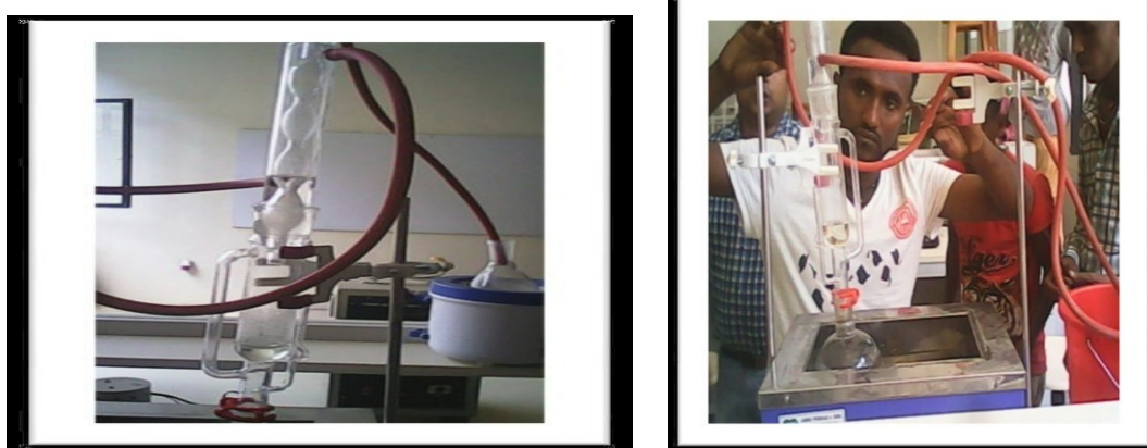
Figure 3.1 Experimental set up for furfural synthesis
