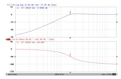
Figure 32. Frequency-domain characteristics of the measured amplitude and phase responses of the first proposed circuit at  $V_{o3}$ .
