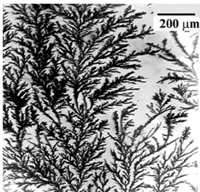
Figure 1. Optical micrograph of a gel-derived \text{Fe}(\text{NO}_3)_3\text{-SiO}_2 film subjected to a d.c. voltage of 5 V and subsequently heated at 400 K for 2 h.
